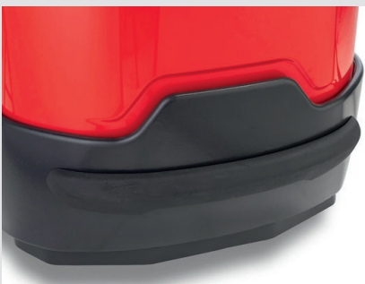
Front casted steel bumper
