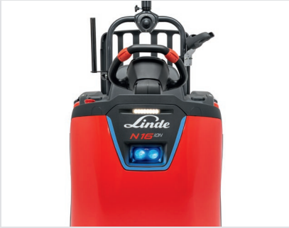
Linde BlueSpot™ and front LED light
